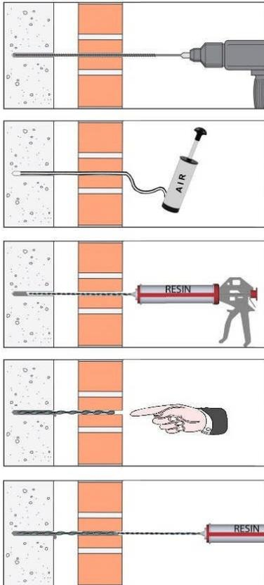
1. Set depth gauge on drill and bore 10mm hole through the near brick leaf and 65-75mm into far leaf material.
