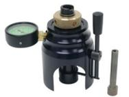
The Thor Helical Tensile Test Unit measures the actual tensile load capacity & is used to generate
